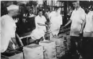
IN MOST foundries pouring technique left much to be desired. Here Mr. Schnur demonstrates proper height from which metal should be poured into gate.
